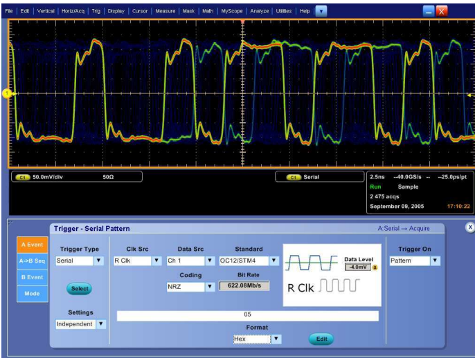
Serial pattern triggering to debug pattern-dependent issues.
