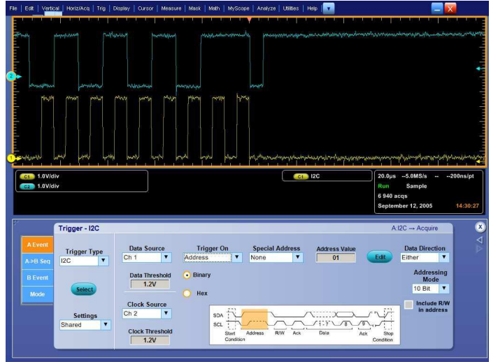
Easily trigger on a specific I2C address.
